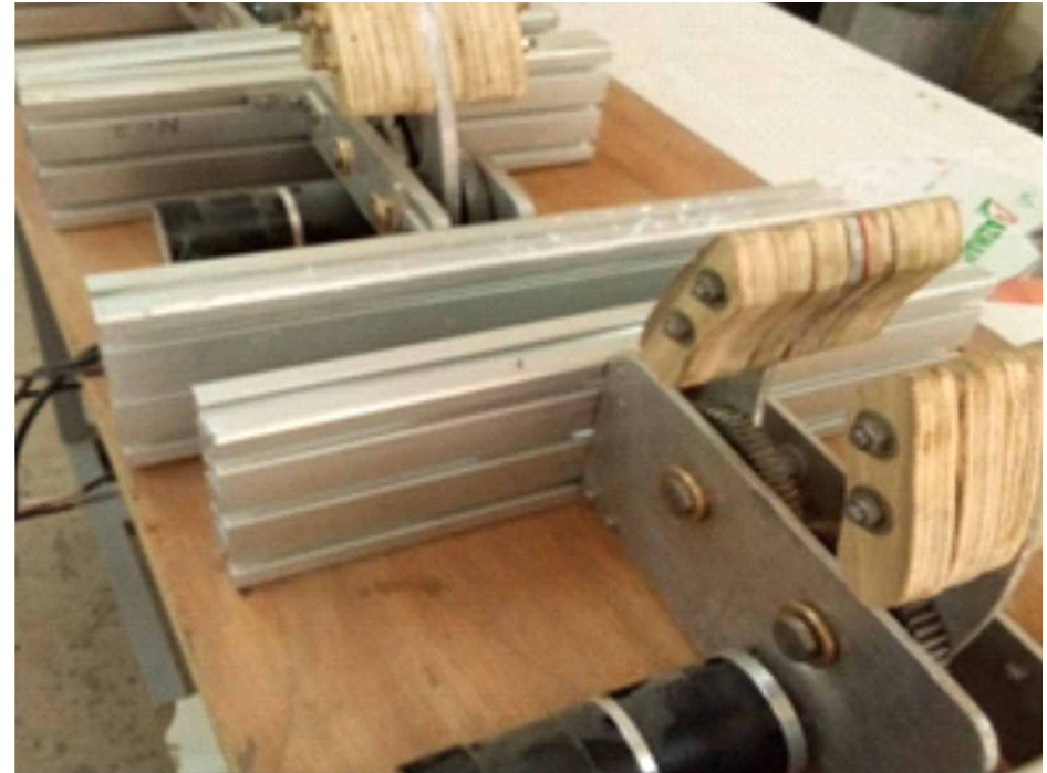
Three units of ventilators under fabrication
